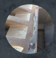
The picture shows a **worn rotor** body. The previous operator didn't change the hammers in time.
