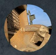
Material built up between the rotor body and side wear plates weren't dealt with. This indicates that the operator didn't open the crusher box for inspection.
