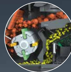
Optimised material flow from the vibro-channel to the main discharge belt
